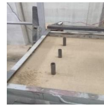
Fig. 3. Pile models after installation.
